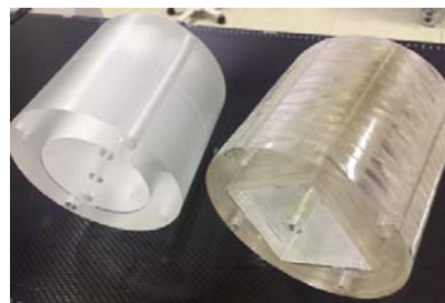
Fig. 3. Standard CTDI phantom (left) and constructed in-house phantom (right).
