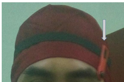
Fig. 1. The EYE-D holder used to measure eye lens dose.
