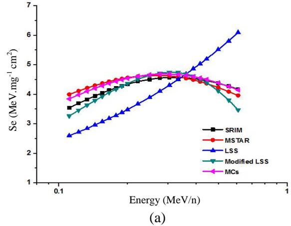
**Fig. 2.** The electronic energy loss as a function of incident ions energy for different heavy ions in Kapton polyimide film  $(C_{22}H_{10}O_5N_2)_n$  polymeric foil. (a) LSS theory and (b) modified LSS theory.
