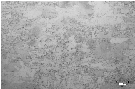
Figure 8. Micrograph of SS-405 rolled sample by 5% strain and then annealed to 550 °C for 24 hours, taken from the sample top surface.
