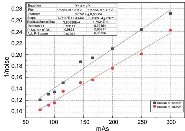
**Fig. 2.** Correlation between image noise and tube current mAs.
