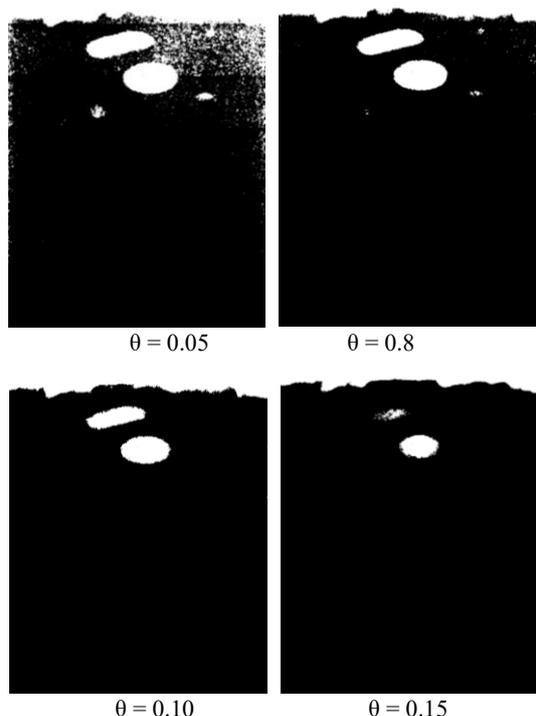
Fig. 3. Binary images of a milk sample after transformation as in Eq. (2) with different values of  $\theta$ .
