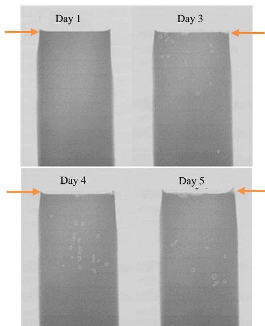
Fig. 4. Radiographic images of a milk sample at different times since air entered the package.
