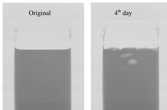
Fig. 2. Radiographic images of a sample in the original state and on the 4<sup>th</sup> day after air infiltration.
