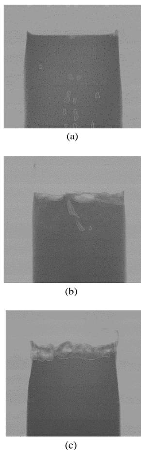
**Fig. 6.** X-ray images of some damaged milk samples. Samples (a); (b); (c) were damaged after 4, 6, and 7 days, respectively, from air-exposed.
