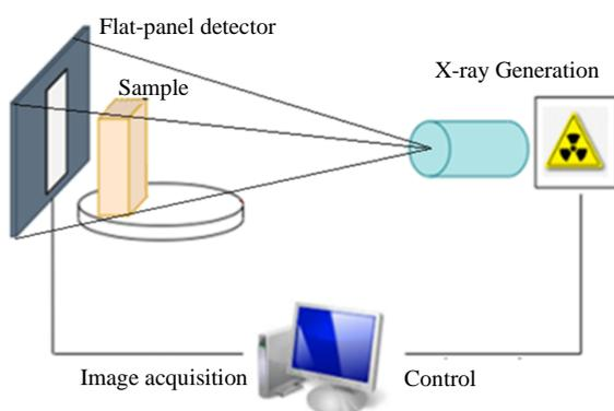
Fig. 1. Diagram of radiographic imaging system.
