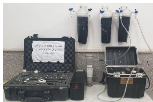
Fig. 3. RAD7 system for measuring radon concentration.
