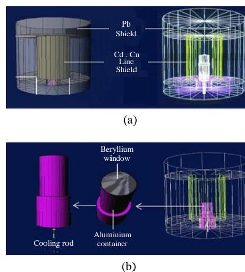
**Fig. 2.** (a) The GMX detector as viewed from outside the Pb shield; (b) The GMX detector as viewed from inside the Pb shield.
