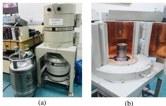
**Fig. 1.** (a) The GMX n-type coaxial HPGe detector inside the standard lead shield and completed with  $\text{LN}_2$  Dewar for nitrogen supply; (b) The lead shield surrounding the GMX detector to reduce the background radiation.
