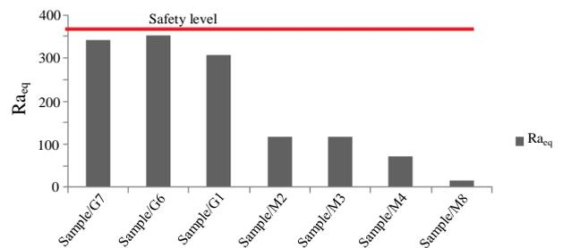
Fig. 5. The radium equivalent activity,  $Ra_{eq}$  for each sample.
