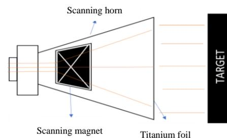
Fig. 1. Scanning Horn Schematic.
