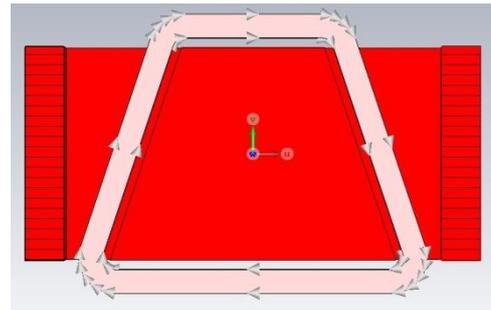
Fig. 2. Cross-sectional image of the scanning horn magnet.
