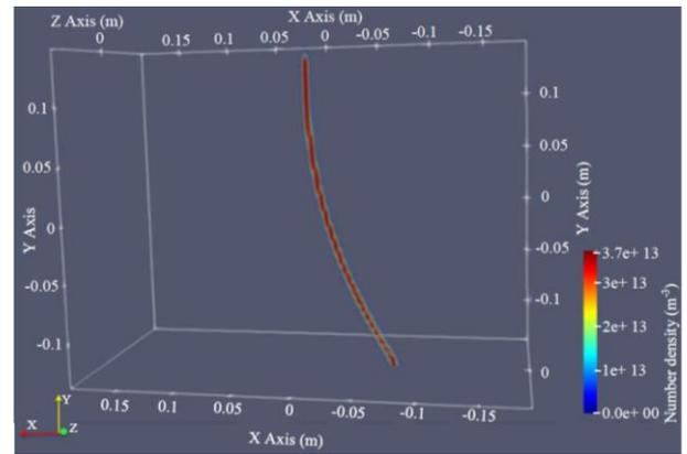
**Fig. 6.** Beam trajectory for scanning horn. The color indicates the number density of particles, with red means the densest region.
