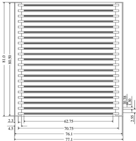
Fig. 2. Dimension of PT INUKI's plate fuel element, in mm [5].
