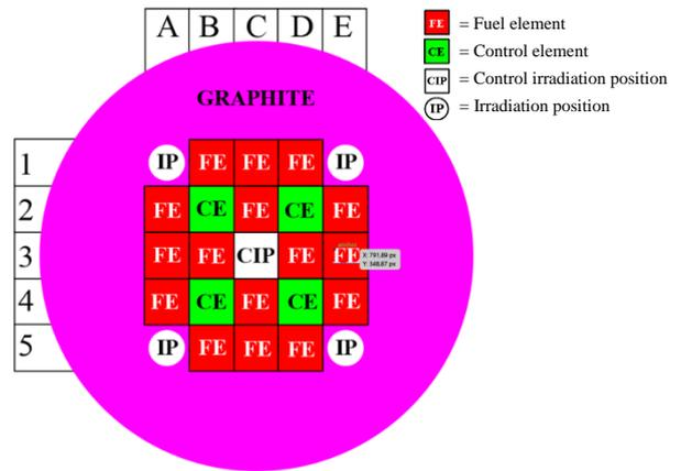
Fig. 1. Reactor core configuration using plate fuel.
