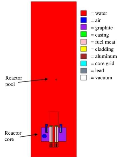
**Fig. 4.** Side view of the TRIGA reactor.
