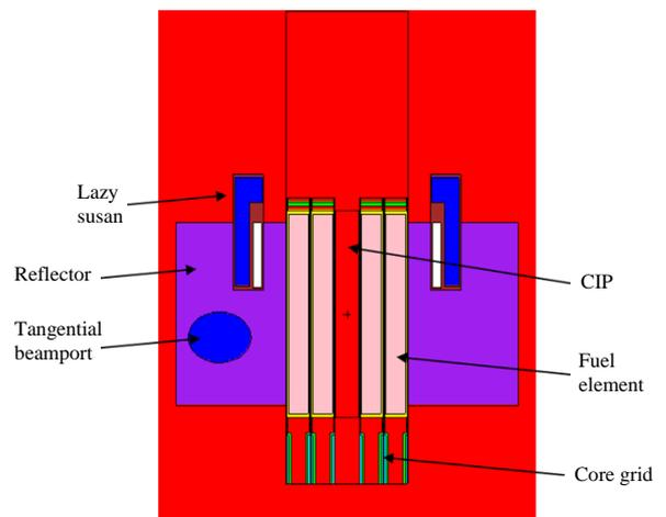
**Fig. 5.** Side view of the reactor core.
