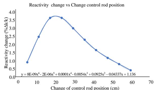
**Fig. 8.** Relation between reactivity change and withdrawn control rod position.
