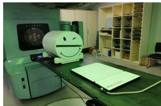
Fig. 2. The Octavius 4D rotational unit and Octavius 729 2D detector array.
