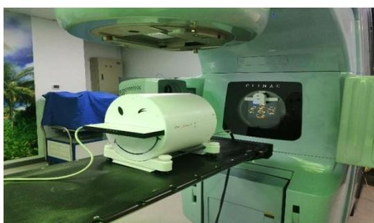
Fig. 3. Standard verification setup, Octavius 4D phantom in facing away from the gantry.
