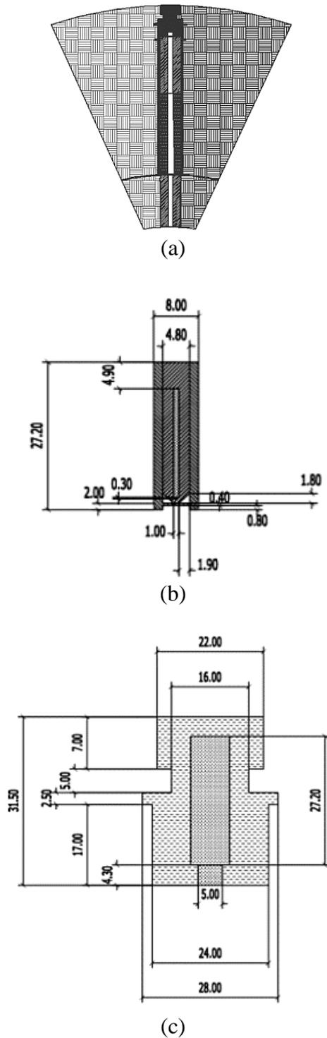
**Fig. 1.** Schematic view of the geometrical models used in the simulation for the different parts of LGK. (a) Entire collimator system for a single source. (b) Capsule involving the radionuclide; (c) Bushing system surrounding the capsule.
