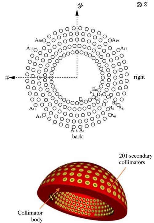
**Fig. 2.** The modeled collimator body shown in PHIG3D.
