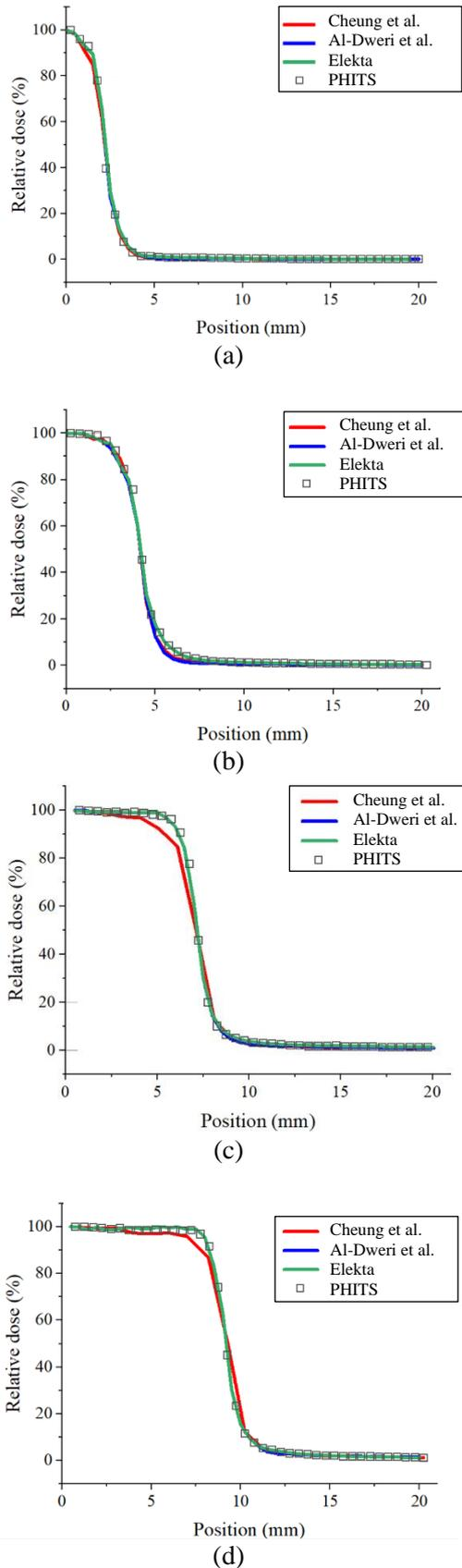
**Fig. 5.** The dose profile (relative to its maximum) as a function of distance from the center axis for various collimator sizes: (a) 4 mm; (b) 8 mm; (c) 14 mm; and (d) 18 mm.
