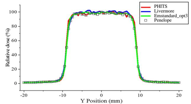
**Fig. 4.** Comparison of PHITS and Geant4 results for 18-mm collimator.
