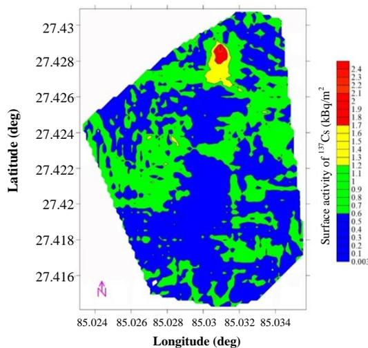
Fig. 4. Contour map showing surface activity of  $^{137}\text{Cs}$  in the environment of Hetauda City.
