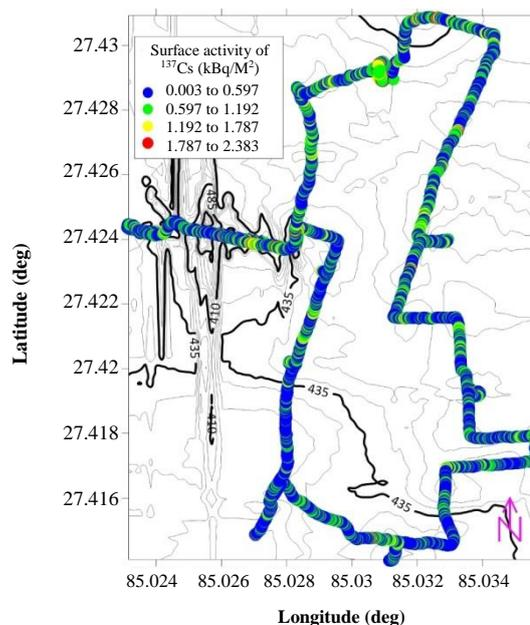
Fig. 3. Spatial distribution of surface activity of  $^{137}\text{Cs}$  in the environment of Hetauda City overlaid on altitude contour.
