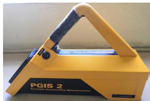
Fig. 2: Gamma ray spectrometer (PGIS 2).
