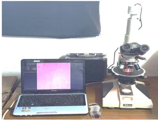
Fig. 6. Scanning the LR-115 SSNTD.
