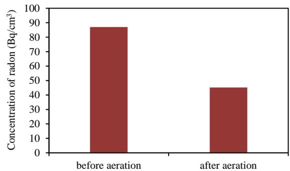
**Fig. 11.** Radon concentration before aeration and after aeration (H2K).
