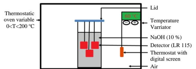
Fig. 5. Conditioning of the chemical etching of the LR-115.
