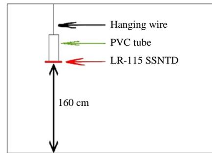
Fig. 4. Radon measurement device with LR-115 SSNTD.
