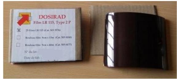
Fig. 3. LR-115 Type 2 solid-state nuclear track detector from Dosirad Laboratory (10 cm × 15 cm).
