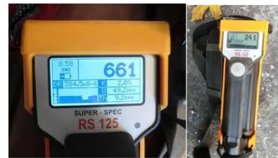
Fig. 3. Gamma-ray spectrometer of RS-125.
