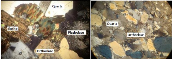
Fig. 10. Thin section image of Menumbing Granite (left) and Mangkol Granite (right) (cross nicol, 120 x magnification).
