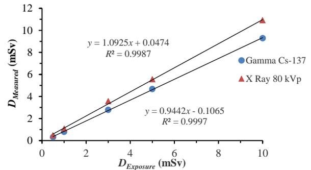
**Fig. 3.** Correlation curve between measured dose and exposure dose on Cs-137 gamma and 80 kVp X-ray irradiation to OSL dosimeter.
