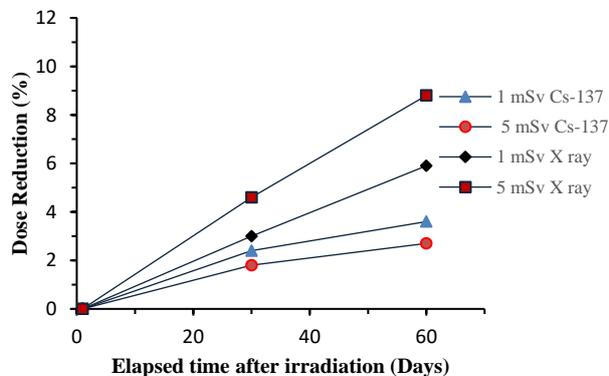
Fig. 5. Fading effect of OSL dosimeter after gamma ray and X-ray irradiation.
