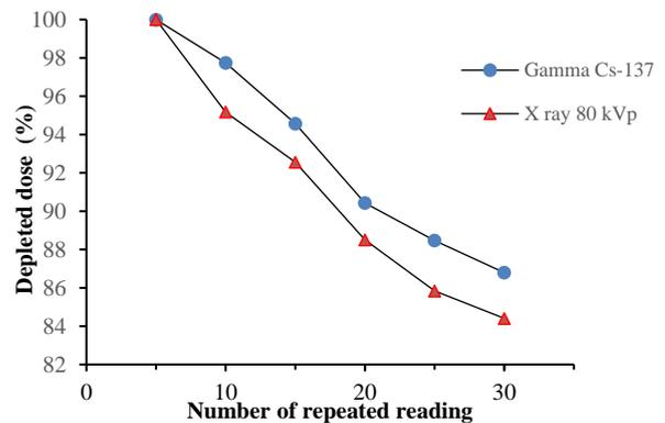
**Fig. 4.** OSL depleted dose for 30 readings obtained by averaging the dose every 5 readings.
