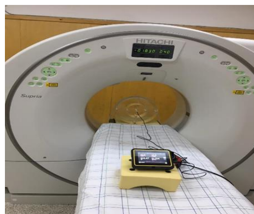
Fig. 1. PMMA phantom with a diameter of 32 cm.
