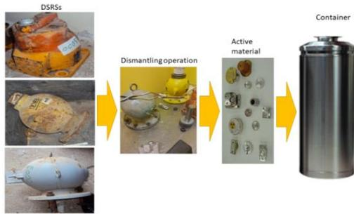
Fig. 1. DSRs dismantling operation principle.
