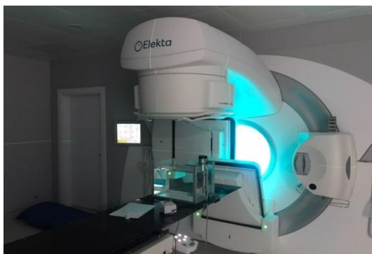
Fig 3. Phantom setup for PDDs measurements.
