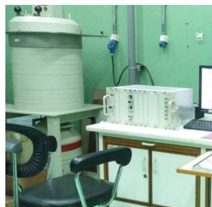
Fig. 3. Table top MCA with HPGe detector.
