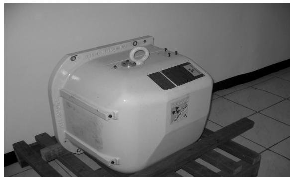
Fig. 2. Container containing radioactive source capsule (spent sealed source).
