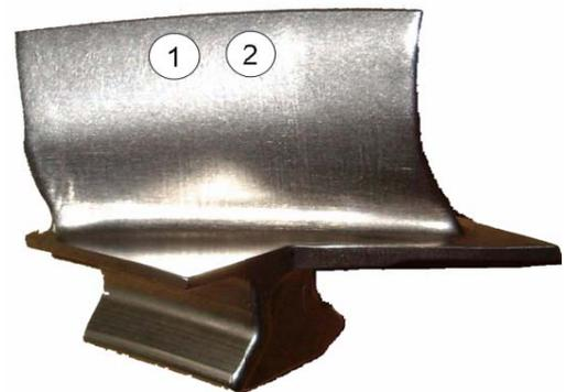
**Fig. 4.** TiAl-turbine blade with dimensions  $6 \times 5 \times 4$  cm<sup>3</sup>. The non-critical beam spot locations 1 and 2 of the measurements in Fig. 5 are indicated.
