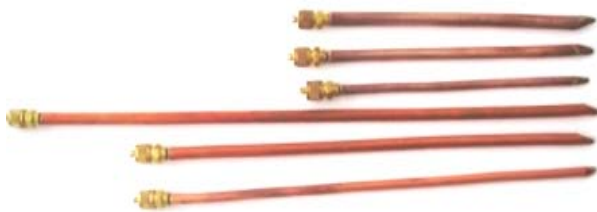
Fig. 4. Copper heat pipe with screen mesh wick.
