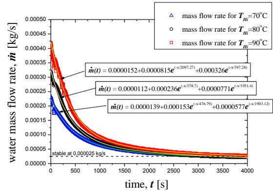
Fig. 7. Water mass flow rate characteristic.
