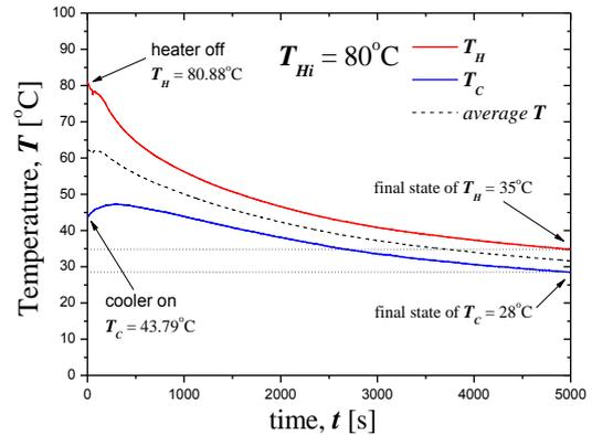
Fig. 4. Temperature measurement in heater and cooler area for initial temperature 80°C.
