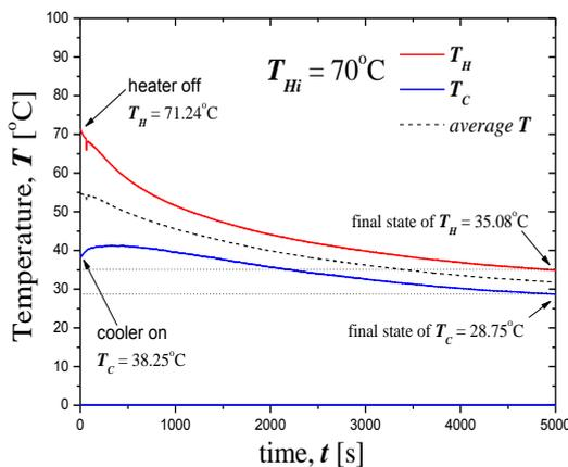
Fig. 3. Temperature measurement in heater and cooler area for initial temperature 70°C.
