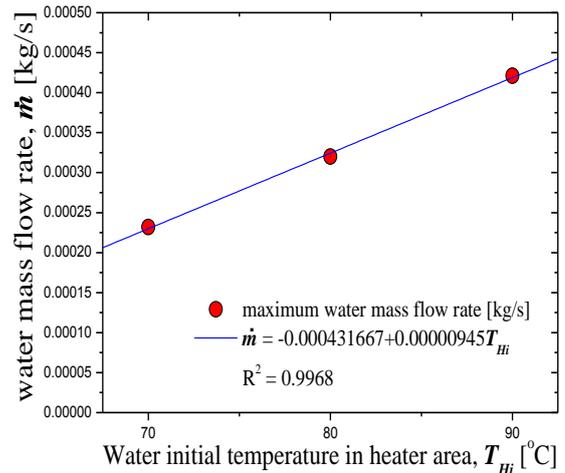
Fig. 10. High water mass flow rate base on initial temperature.
