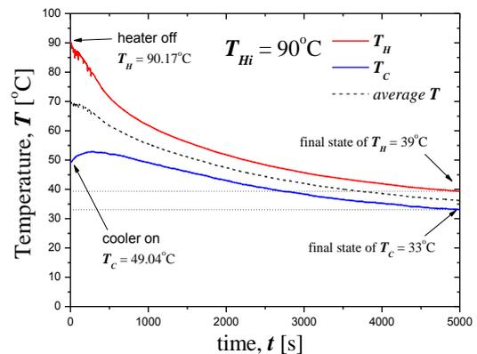
Fig. 5. Temperature measurement in heater and cooler area for initial temperature 90°C.
