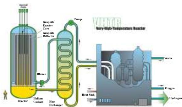
Fig. 1. Very High Temperature Reactor [3].
