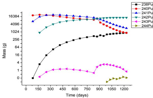
**Fig. 4(b).** Plutonium isotopes variation in the hybrid system ( $^{238}\text{Pu}$ ,  $^{240}\text{Pu}$ ,  $^{241}\text{Pu}$ ,  $^{242}\text{Pu}$ ,  $^{243}\text{Pu}$  and  $^{244}\text{Pu}$ ) in  $^{232}\text{Th}$ - $^{239}\text{Pu}$  cycle.
