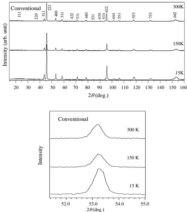
**Fig. 5.** Neutron diffraction patterns taken from HRPD-HANARO of the spinel-type  $\text{LiMn}_2\text{O}_4$  synthesized with an initial molar ratio of  $\text{Li}/\text{Mn} = 0.50$  by conventional method and annealed at  $800^\circ\text{C}$  for 4 hours in  $\text{O}_2$  then cooled with cooling rate of  $60^\circ\text{C}/\text{h}$ . (a) whole pattern and (b) (400) peaks.
