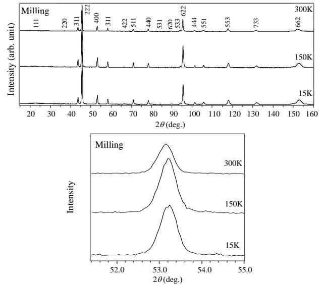
**Fig. 6.** Neutron diffraction patterns taken from HRPD-HANARO of the spinel-type  $\text{LiMn}_2\text{O}_4$  synthesized with an initial molar ratio of  $\text{Li}/\text{Mn} = 0.50$  by MA method and annealed at  $800^\circ\text{C}$  for 4 hours in  $\text{O}_2$  then cooled with cooling rate of  $60^\circ\text{C}/\text{h}$ . (a) whole pattern and (b) (400) peaks.
