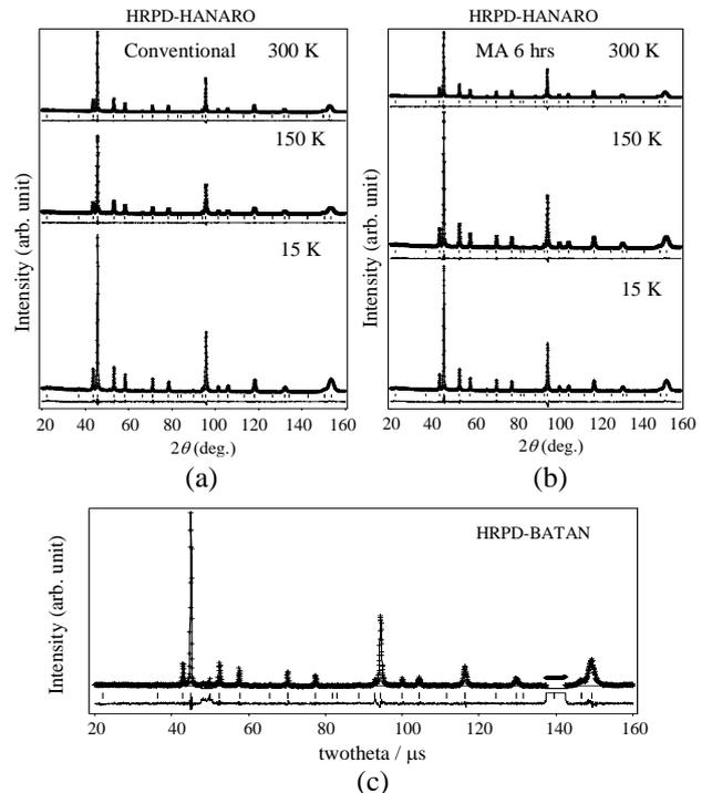
**Fig. 7.** Rietveld refinement patterns for neutron diffraction measurement at 15K, 150K and 300K (HRPD-HANARO) of spinel  $\text{LiMn}_2\text{O}_4$  synthesized by a) conventional and b) MA methods and annealed at  $800^\circ\text{C}$  in  $\text{O}_2$ . (c) commercial/standard  $\text{LiMn}_2\text{O}_4$  measured at 300K (HRPD-BATAN).
