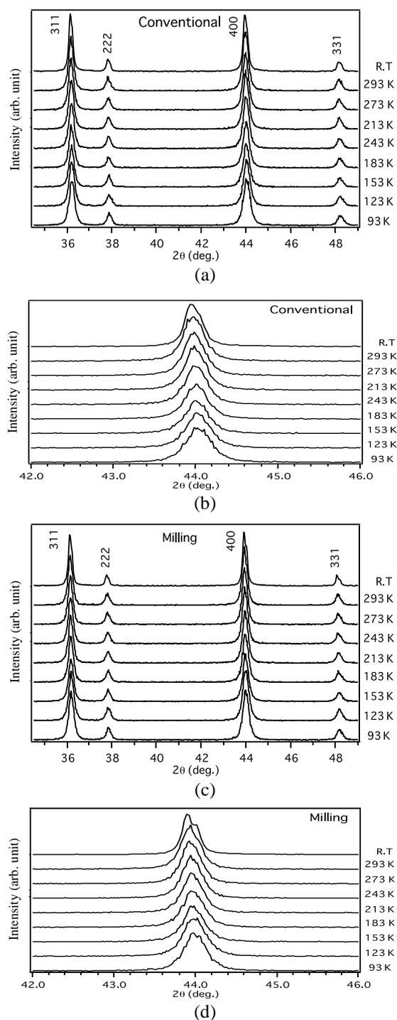
**Fig. 3.** XRD patterns of the spinel-type  $\text{LiMn}_2\text{O}_4$  synthesized with an initial molar ratio of  $\text{Li}/\text{Mn} = 0.50$  by conventional method (a) and (b) and MA method for 6 hours (c) and (d) and annealed at 800 °C for 4 hours in  $\text{O}_2$  then cooled with cooling rate of 60 °C/h. (a) and (c)  $2\theta$  region from 34.5 ° to 49 ° and (b) and (d) peaks of (400) plane.
