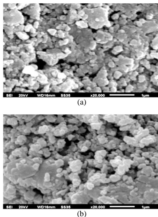
**Fig. 1.** SEM micrograph of the spinel-type  $\text{LiMn}_2\text{O}_4$  synthesized with an initial molar ratio of  $\text{Li}/\text{Mn} = 0.50$  (a) after MA for 6 hours and (b) conventionally prepared, and after annealed at 800 °C for 4 hours in  $\text{O}_2$  then cooled with cooling rate of 60 °C/h.
