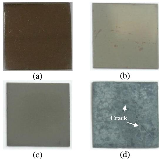
Fig. 3. Appearances of Fe-Cr steel (a) before and after high temperature oxidation test at (b) 1000 K, (c) 1100 K and (d) 1200 K for 72 ks.
