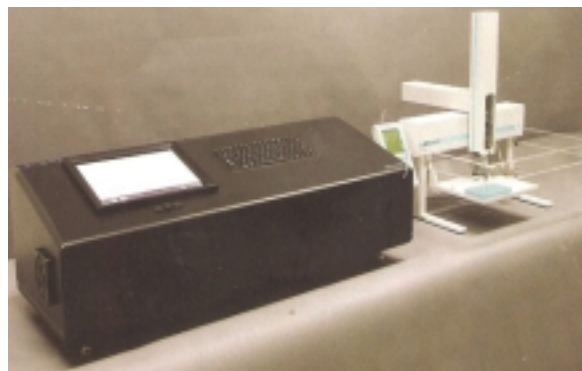
Fig. 1. LGR DLT-100 liquid – water stable isotope instrument and CTC LC-PAL liquid auto sampler.
