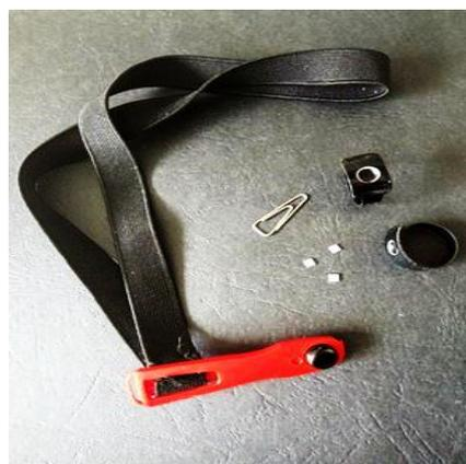
**Fig. 1.** The 'eye-D' holder used to measure eye lens dose (left) and the ring holder to measure extremity dose (right).
