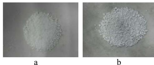
**Fig. 1.** The sulfated zirconia: (a) prior to calcination (b) after calcination.
