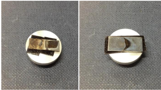
Fig. 1. A contamination in the vacuum system has invalidated specimens irradiated at 380 °C.
